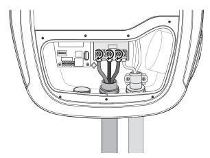
Figure 10. Securing the Input Cable
