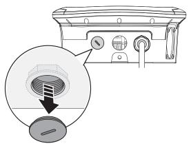
Figure 11. Removing the Water Proof Cap
