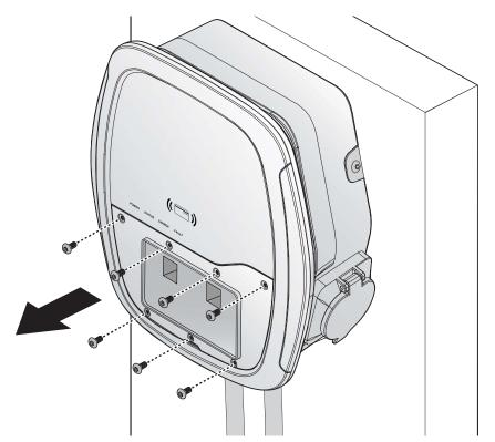
Figure 6. Removing a Compartment Cover
