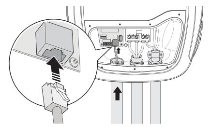
Figure 14. Installing an Ethernet Cable
