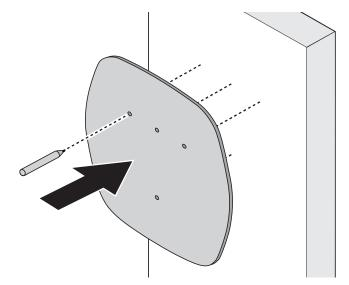
Figure 3. Template for Marking the Screw Locations
