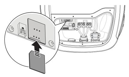
Figure 15. Installing a SIM Card
