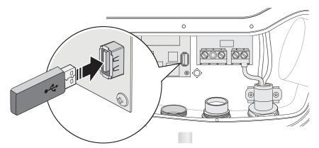
Figure 21. Inserting a USB Flash Drive
