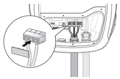
Figure 16. Installing a Terminal Cover
