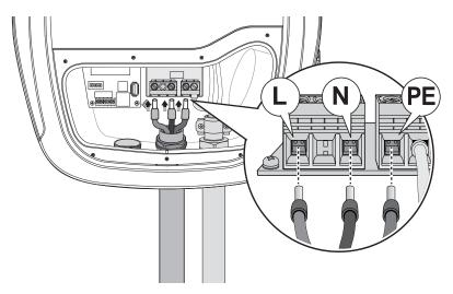
Figure 9. Connecting the Terminal Connector
