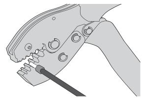
Figure 8. Crimping a Terminal End
