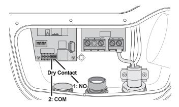
Figure 12. Dry Contact Wiring Connection - 3G Model
