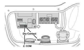
Figure 13. Dry Contact Wiring Connection - WiFi Model
