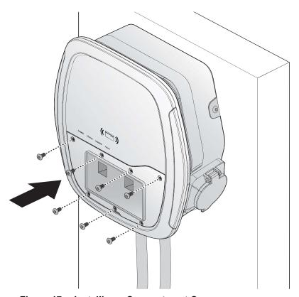
Figure 17. Installing a Compartment Cover
